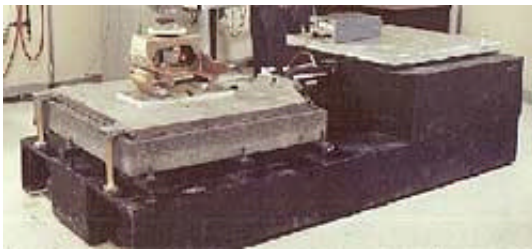
954; 3 ft x 6 ft x 11 in with step for servo-hydraulic shaker
