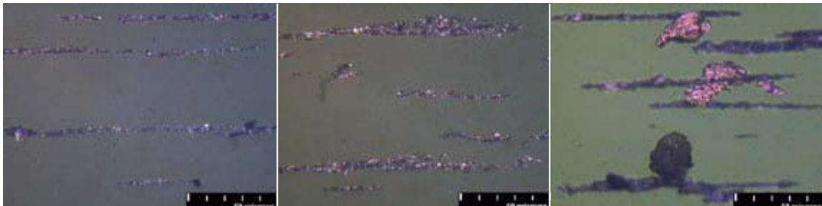
Figure 7c, Photographs Showing Fine Rubbing Wear During Normal Running
