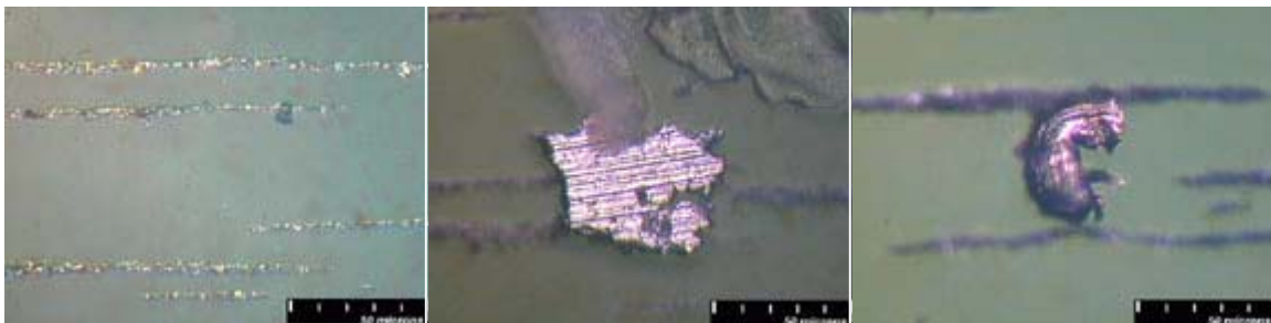
Figure 8c, Photographs Showing Fine Rubbing Wear and the Occasional Larger Particle
