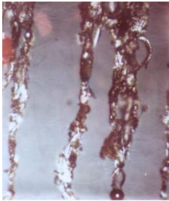
Figure 4, Ferrogram Showing Cutting Wear and Weld Beads
