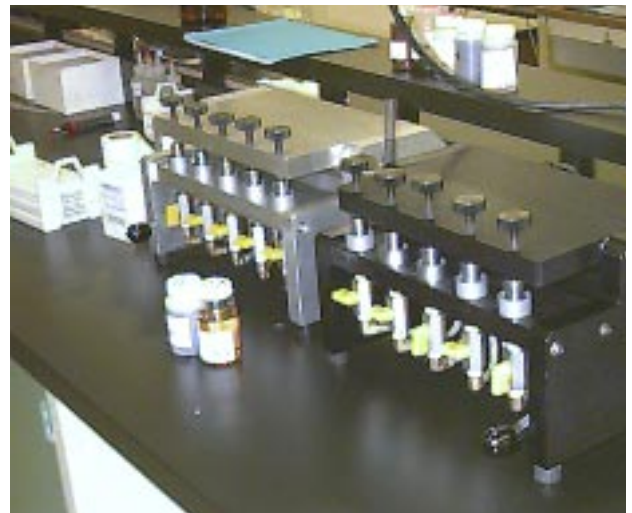
Figure 2, Multi-station RFS Sample Preparation Fixture
