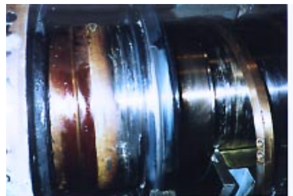
Figure 8, Slinger Ring Assembly Showing Abnormal Wear
