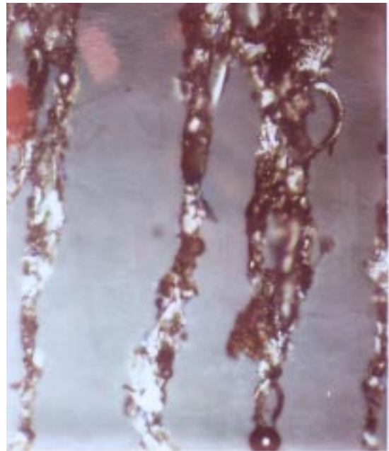
Figure 4, Ferrogram Showing Cutting Wear and Weld Beads
