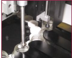
solvent, interspersed with air gaps, is also pumped through the sipper, LNF tubing and the LNF flow cell to wash away traces of the previous sample. The procedure is repeated until up to 24 samples are analyzed and processed. Sensors monitor the complete process, step by step, and shut down the system if an error occurs.
