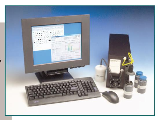
"The LaserNet Fines-C (LNF-C) uses laser imaging techniques and advanced image processing software to identify the type, rate of production, and severity of mechanical faults by measuring the size distribution, rate of progression, and shape features of wear debris in lubricating fluids."
