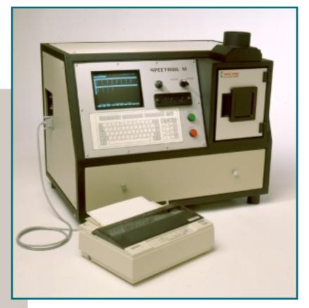
"...for rapid on-site trace metal analysis of liquid fuels used in liquid-fired gas turbines and diesel engines"
