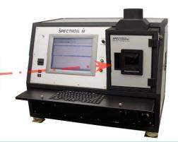
monitored by expanding the particle detection capability of the RDE technique. It is sometimes also used to screen samples for more time consuming analyses such as ferrography.
