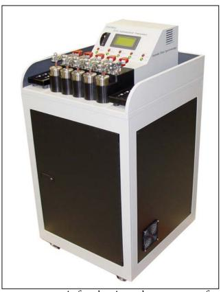
electrode preparation fixture, vacuum/pressure pump, a reservoir for cleaning solvent, a sump for waste oil, and electrode clamp assemblies. It requires only external electrical power for operation and uses only environmentally friendly solvents. The entire system is on casters and can be easily transported.
