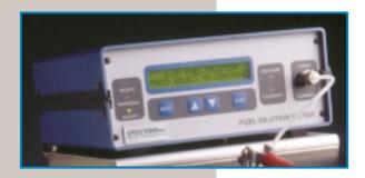
Operating instructions are displayed on the LCD screen and functions are selected from the menu by pressing a single key.
